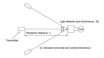
Fig. 2 Standard optical system
